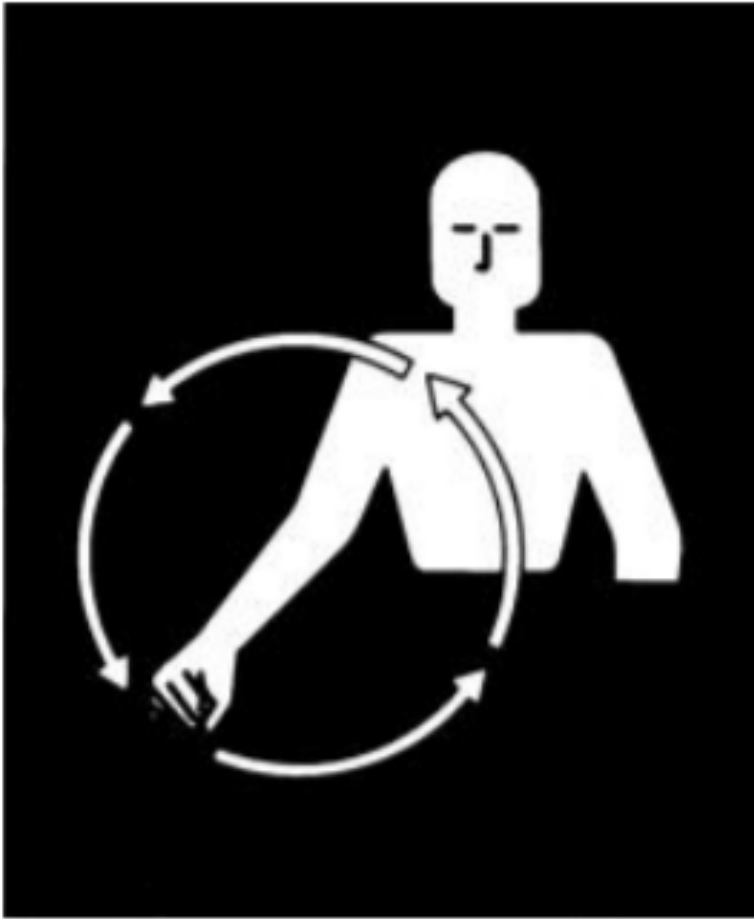
Figure 8 – START THE ENGINE — Simulate cranking of vehicles by moving arm in a circular motion at waist level.
