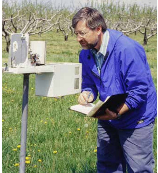
Jim Travis examining a leaf wetness device for determining apple scab infection periods
