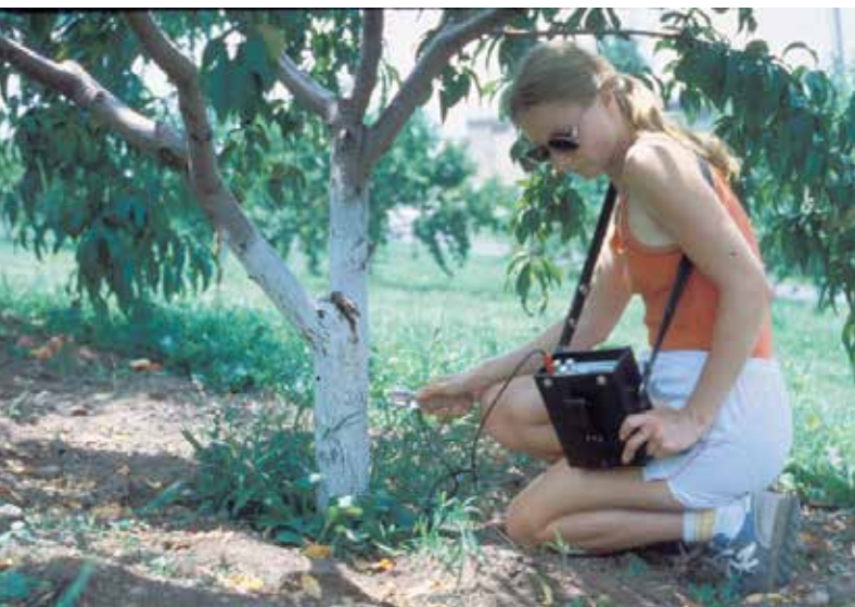
Debbie Breth, graduate student of Jim Travis and Larry Hull, measures electrical conductivity of peach trees inoculated with cytospora canker and lesser peach tree borers
