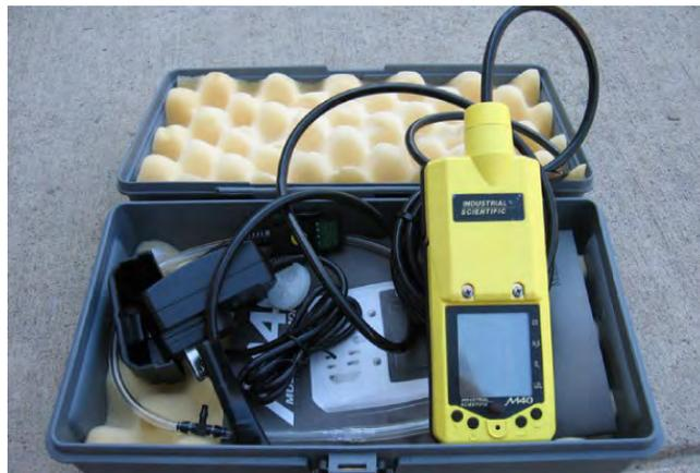
Figure 3. Hand-held, portable multi-gas monitors measure most of the manure gases and oxygen levels.
