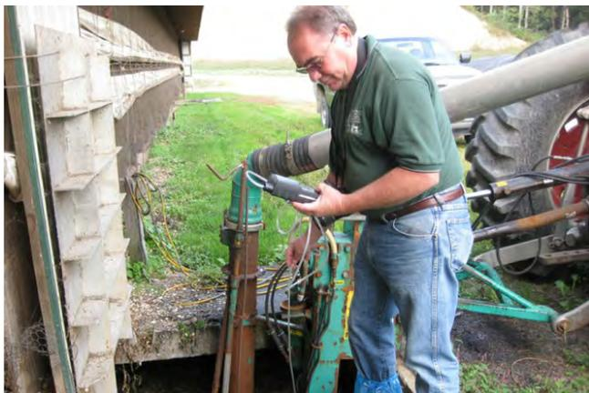
Figure 4. Always remain outside the manure storage facility when taking initial gas measurements.
