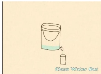
Figure 2: A Penn State team proposed a solution to the problem of water-borne illnesses caused by contaminated drinking water. A ceramic water filter using silver ions to disrupt microbial activity can turn unsafe water into drinkable water.
