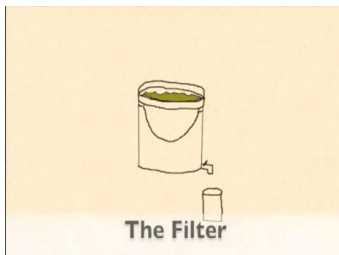
Figure 2: A Penn State team proposed a solution to the problem of water-borne illnesses caused by contaminated drinking water. A ceramic water filter using silver ions to disrupt microbial activity can turn unsafe water into drinkable water.
