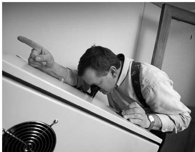
▲ Research technician Pat Topper detects an odor and signals the operator of the olfactometer in the college's Odor Laboratory.
